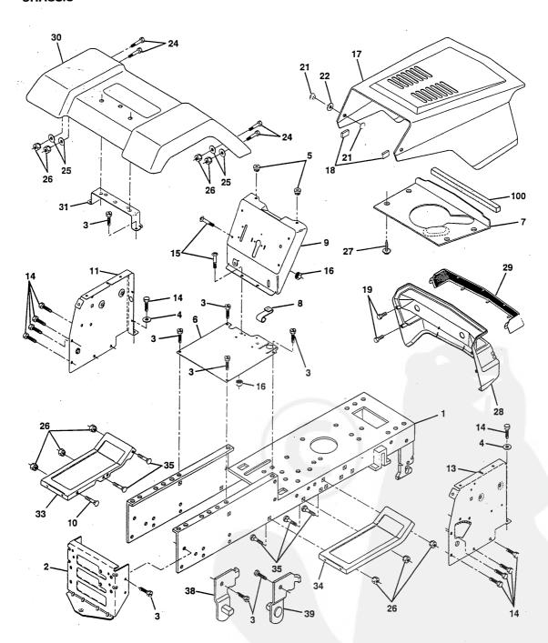
TRACTEUR -- NO. DE MODÈLE BL1542LTDHA, NO. DE PRODUIT 954 81 00-11 CHÂSSIS
