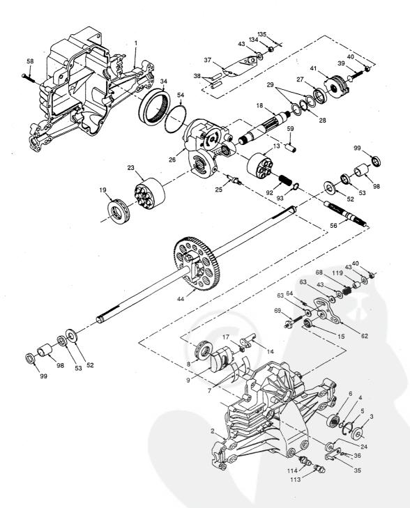
TRACTEUR -- NO. DE MODÈLE BL1542LTDHA, NO. DE PRODUIT 954 81 00-11 TRANSMISSION DE HYDRO-GEAR - 310-0500
