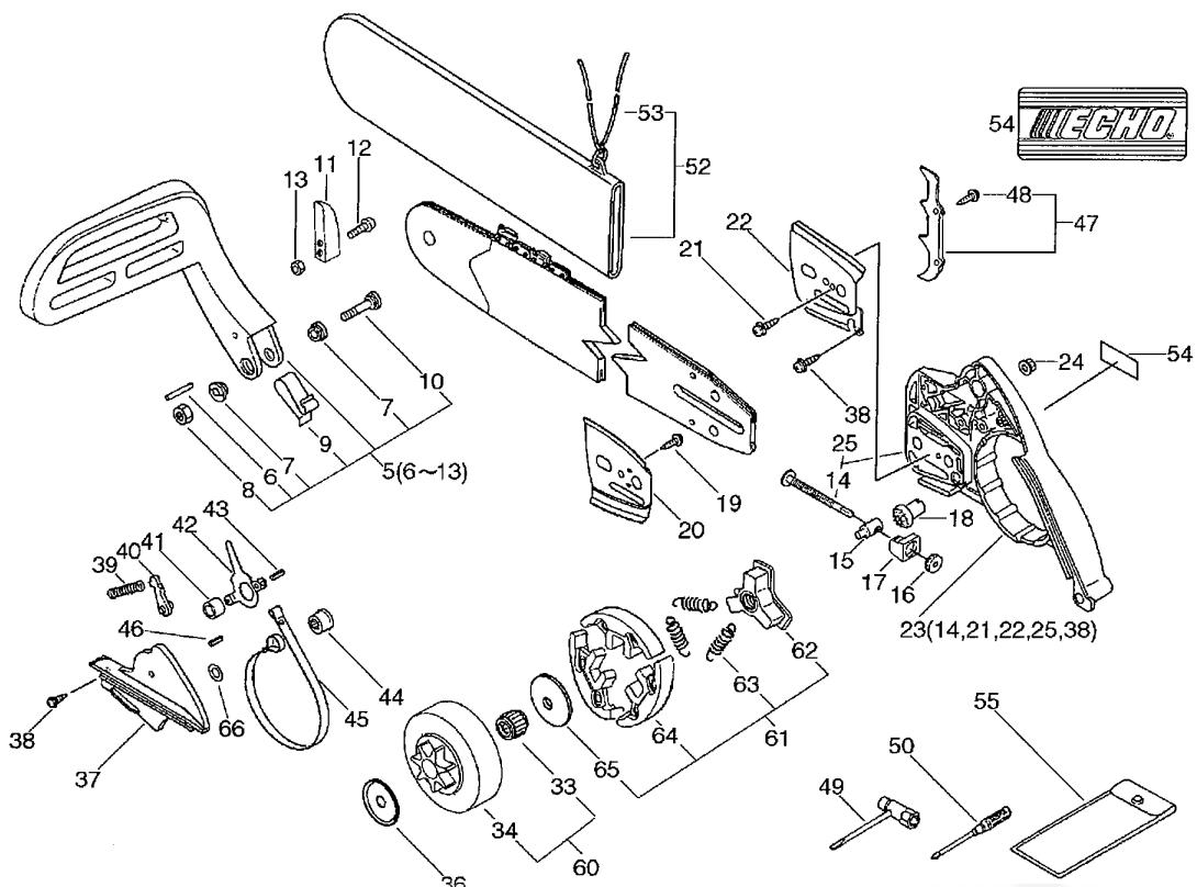
Clutch, Sprocket, Tools(Sr/Nr 36020671 and after)
