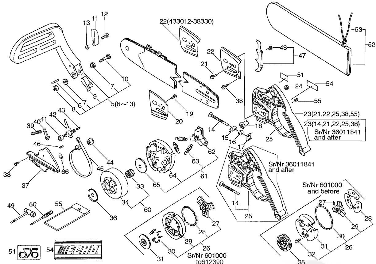
Clutch, Sprocket, Tools(Sr/Nr 36020670 and before)
